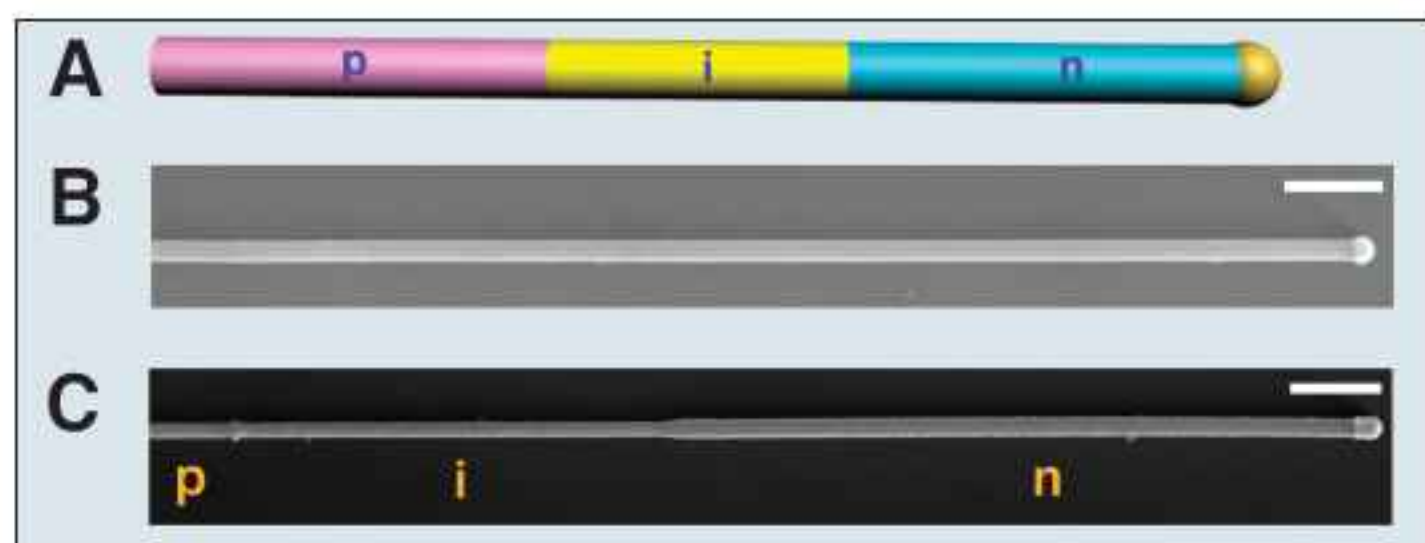
Figure 4. Axial p-i-n Si NWs scheme (A), and SEMs before (B) and after a selective wet etching process (C) that shows p and i regions due to faster etch rate.
